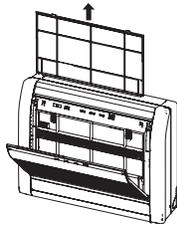
2. Install the Air cleaning filter set (set of 2).
