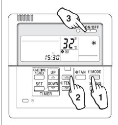
① On a sunny day, keep the system running for half a day in the FAN mode to dry it up inside.
