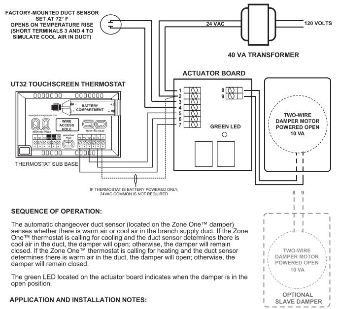
The UT32 thermostat can control up to three Zone One dampers wired in parallel.
