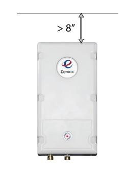
**3.** Remove the cover and fasten to the wall using the four mounting holes at each corner of the back plate. Replace the cover.
