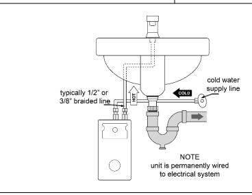
**4.** Open the hot water faucet and run water for a minimum of 60 seconds and until the flow is continuous and free of air pockets. Close the faucet and install the aerator (if supplied).
