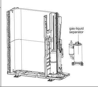
20. Remove supporting board and supporting board sub-assy
