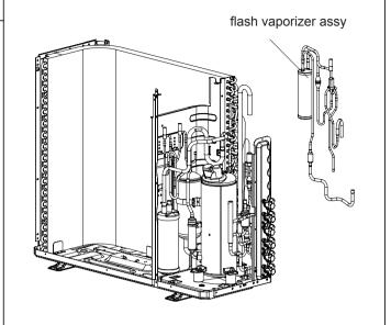
11. Remove electromagnetic valve sub-assy and inhalation tube sub-assy
