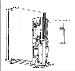
19. Remove gas-liquid separator
