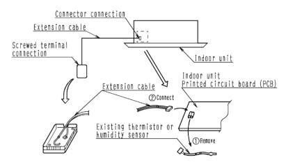
KRCS01-2UA includes Wiring Harness Adaptor WHKRCS01-4-2A that connects Extension Cable KRCS01-4B to the X4A connector on the FXTQ TA PCB:
