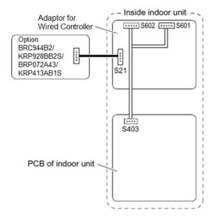
• Connects to BRC944B2 and KRP928BB2S together
