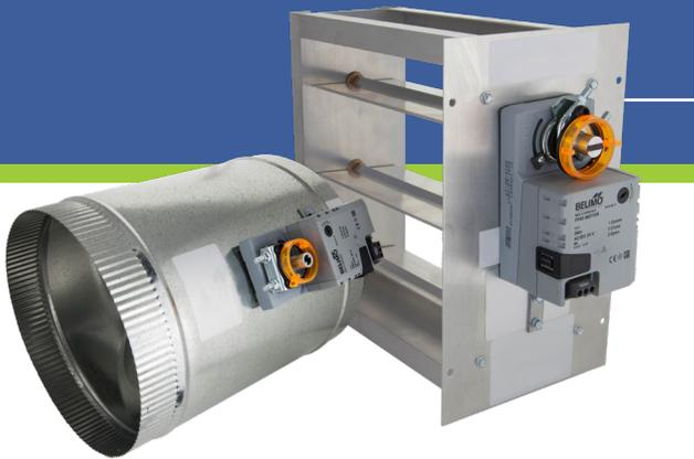
The MD Series dampers are perfect for use with most zoning systems and recommended for use with our ESP zone panels. These dampers are shipped complete and ready for installation. The MD Series dampers can be installed in any position. They are rated for duct systems less than 1.0" WC. The MD Series dampers have a simple adjustment for setting the minimum position.
