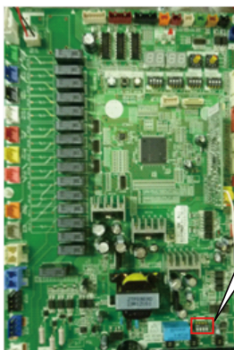
The 4th switch in SET5 DipSW of Outdoor unit PCB (On: Enable, Off: Disable)
