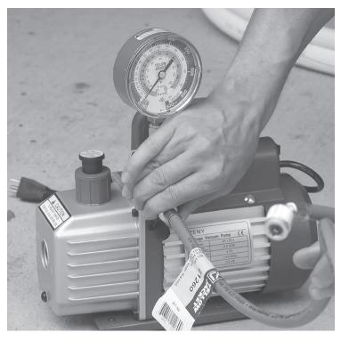
**STEP 9** On the vacuum pump, thread on the 60" length of flexible hi-pressure hose to hand tight on the other side of the low-pressure tee.
