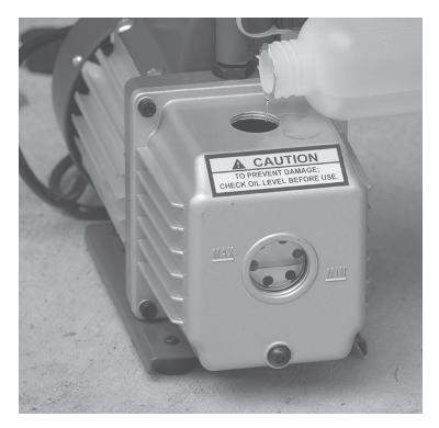
**STEP 6** Prepare the vacuum pump by unscrewing the oil reservoir cap and filling with the pump oil. Use the sight glass on the side of the pump to fill to the indicator lines.
