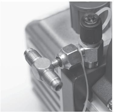
**STEP 7** On the vacuum pump, remove the inlet cover and thread on the low-pressure tee to hand tight.
