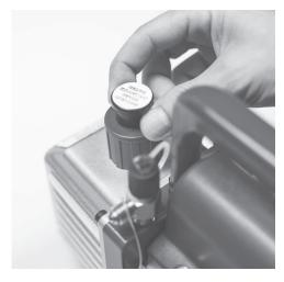
**STEP 12** On the vacuum, remove the exhaust cap that says "REMOVE EXHAUST CAP BEFORE OPERATING". With the vacuum pump plugged into AC power, turn on the pump and allow to run. You will see mist coming from the exhaust port.
