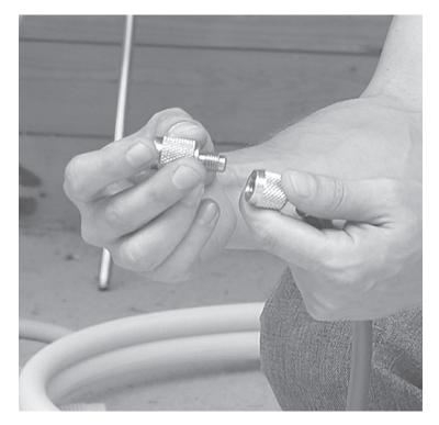
**STEP 10** Thread on the adapter to the flexible hi-pressure tubing.
