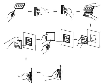
Figure 2-5-2 Installation of wired controller
