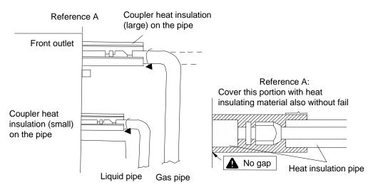
Stick coupler heat insulation (large and small) to the place where connecting pipes.
