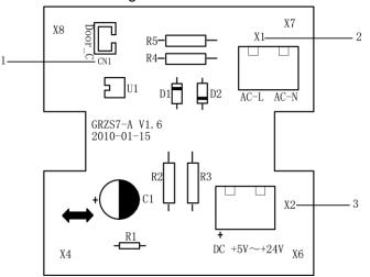
Figure 2-7-6 Illustration of door control port
