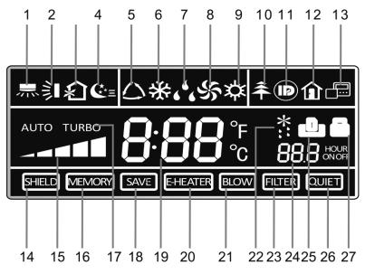
Figure 2-3-2 LCD display of wired controller
