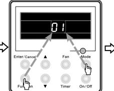
Press Function and Mode buttons to enter address setting
