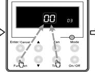
Press Function and Timer buttons at the same time for 5s to enter the interface of parameter setting
