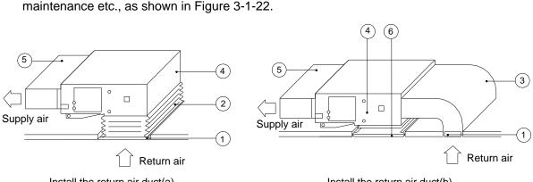
Install the return air duct(a)
