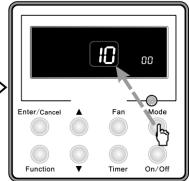
Press Mode button to adjust to "10" in temperature displaying zone and enter selection of centralized controller or long-distance control.
