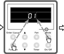
Press Function and Mode buttons to enter address setting
