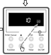
Press Enter/Cancel button to save and exit setting; now, the wired controller address is long-distance control address
