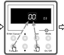
Press Function and Timer buttons at the same time for 5s to enter the interface of parameter setting
