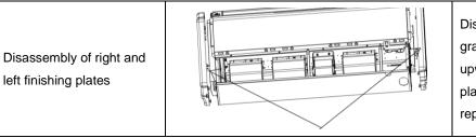
Disassemble the screws as shown in the graph with screwdriver and then push upward to remove the right and left finishing plates. (As is shown in the graph, arrow represents the position of screws.)
