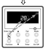
Press Enter/Cancel button to confirm and exit setting interface; If slave wired controller is set, the corresponding icon will be displayed
