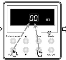
Press Function and Timer buttons at the same time for 5s to enter the interface of parameter setting
