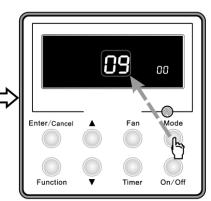
Press Mode button to adjust to "09" in temperature displaying zone and enter setting of human sensitive function \_\_\_\_
