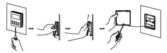
Figure 2-5-3 Removal of wired controller
