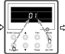
Press Function and Mode buttons at the same time to enter setting of address
