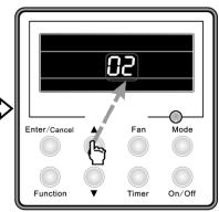
Press ▲ or ▼ button to adjust the address sequence
