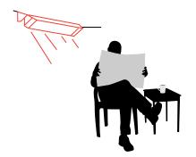
Install fixture to heat the area from the "cold side" if possible. This helps compensate for increased body heat losses due to exposure. Warm floors reradiate heat. Warmer air rises from floor. Some heat reflects from floor. Mounting a heater
